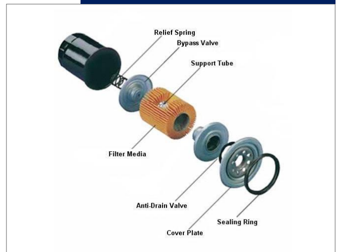
Exploded view – Oil filter
